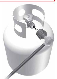
▲ Any fuel supply cylinder used must be constructed and marked in accordance with specifications for propane cylinders of the U.S. Department of Transportation (DOT) CFR 49, or CAN/CSA B339. The appliances is to be used only with the 20 pound, vertical standing vapor withdrawal type tank.
